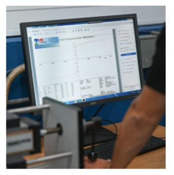
All requirements of the magnetic properties of a material, such as it's coercivity field strength, permeability, etc. can be monitored with our Remagraph and if necessary, could also be documented.
