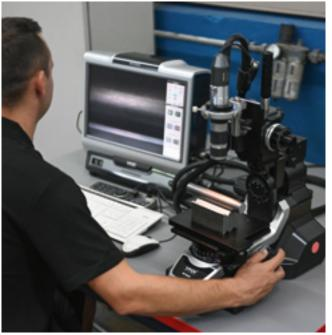
Experienced personnel conducts research studies of structure and degree of purity using a microscope with magnification of up to 1000-fold.
