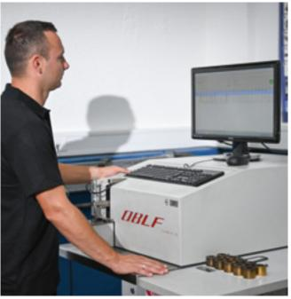
Samples are taken from each BESSEY steel production lot. These are compared using an emission spectrometer on their chemical analysis (up to 20 material identifying elements) with the quality used as well as the desired quality, and documented. Thus, an accurate batch assignment is ensured.
