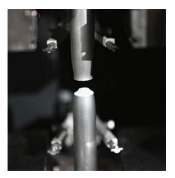
With a 400 kN tear machine, strength and elongation values are determined in our company for all our products and attested upon request.
